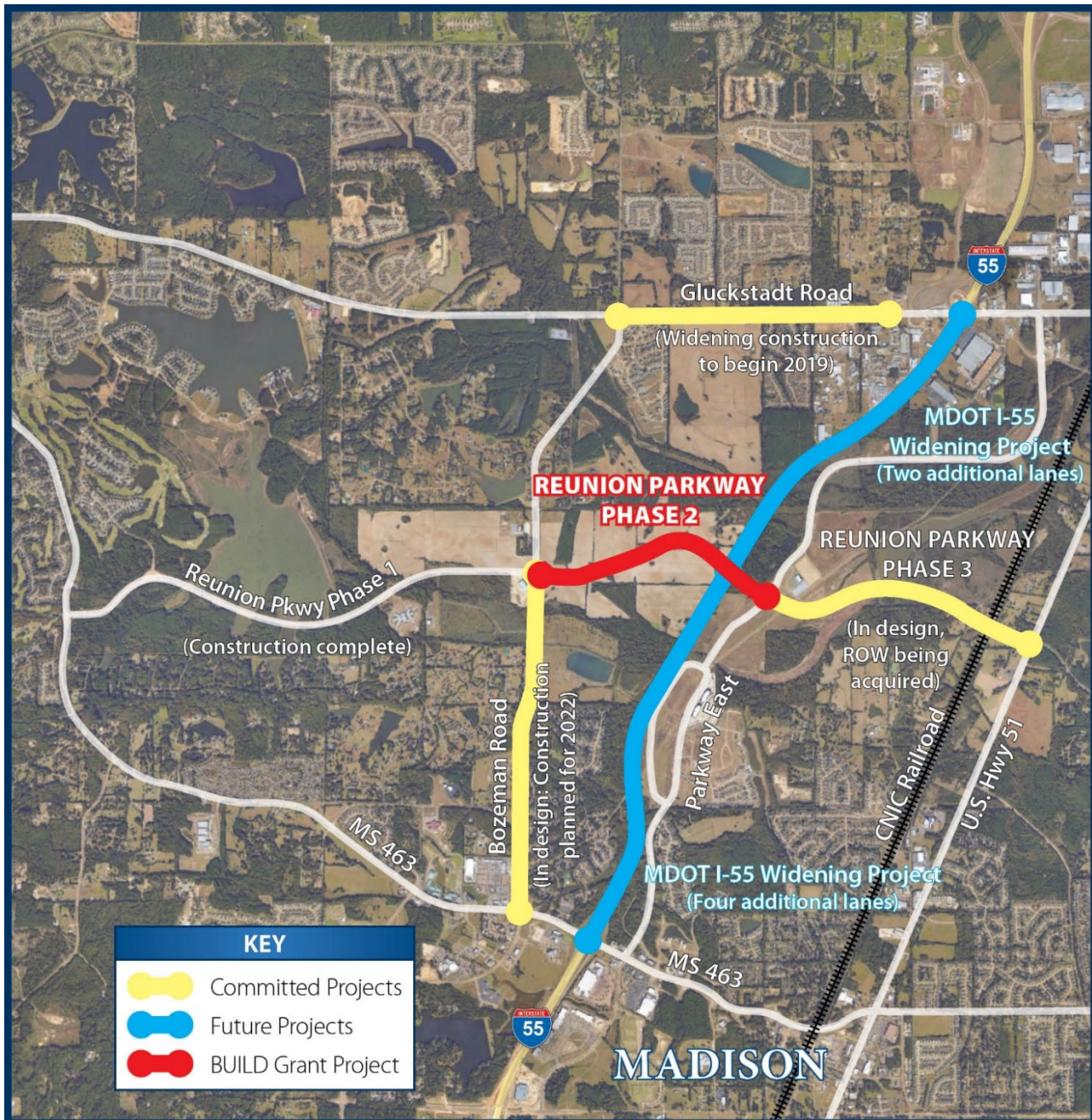
Figure 4: Connections to Existing and Future Transportation Infrastructure
